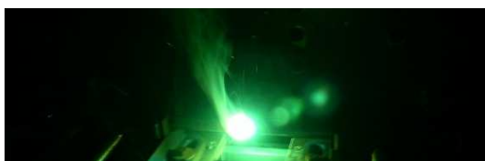
Fig. 12 DC arc, Fe-electrodes, d = 5 mm, U_a = 35 V, I_a = 119 A
