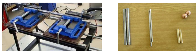
Fig. 11 Electrodes system and various electrodes for measuring on the DC electric arc
