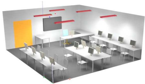
Fig.5: Modelling of artificial lighting (software Dialux) – 2nd model with interior equipment [4]
