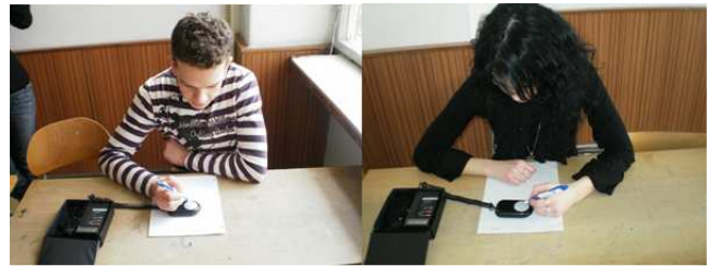
Fig. 11: Measurement of lighting of work area for right-handed and left-handed people
