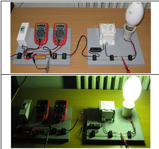
Fig. 7. The arrangement of block for measurement on the mercury discharge lamp
